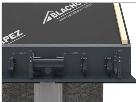
Lowest mounting point of the bracket with the outlet.
